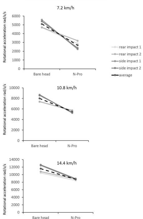
Figure 4 Measured rotational acceleration (rad/s/s) at rear and side of headforms at three different test velocities. values shown are for bare headforms and headforms with N-Pro.
